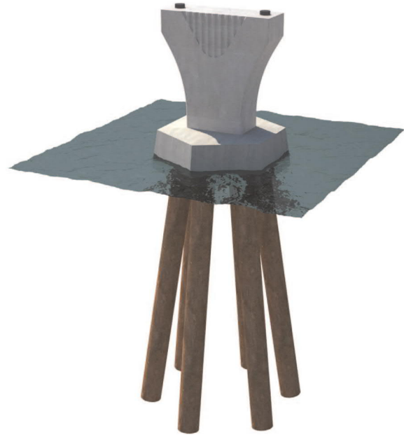
Figure 3. Pier, pile cap and pile arrangement.
